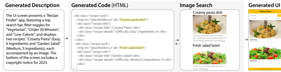
Fig. 3: An example of a generated UI description with the corresponding generated code and generated UI. In the Production phase, our pipeline extracts alternative text and placeholder image link and uses Bing Search API or DALL·E to get a link or image to replace the placeholder.
