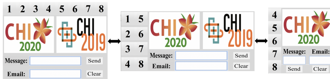
Figure 1. ORCSolver is able to adapt a layout between different sizes and orientations at near-interactive rates, based on a single layout specification. The layout is adjusted to fit the aspect ratio, and the optional “CHI2019” logo and buttons 1, 2, 3 are automatically removed as space gets scarce.
